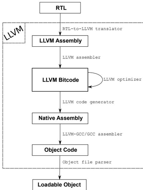
Figure 5: The LLVM component of HiPE’s pipeline.
