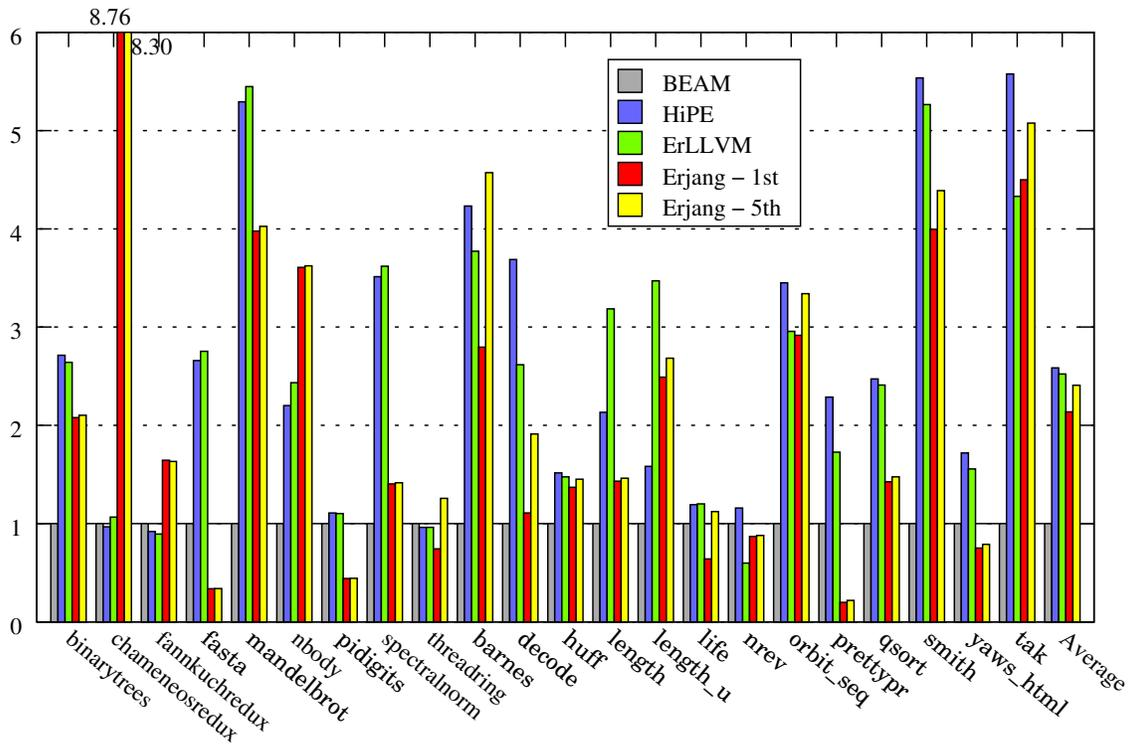
Figure 9: Speedups on x86\_64 (normalized to BEAM).
