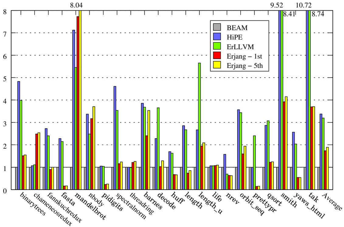
Figure 10: Speedups on x86 (normalized to BEAM).
